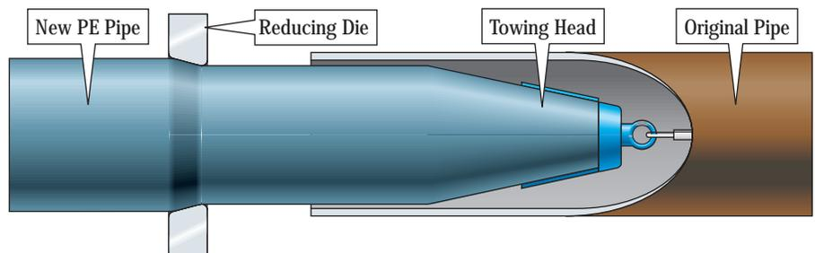
▶ The PE pipe is reduced slightly during the installation process. This allows it to be pulled easily through an existing pipeline. Within a short time after installation, the PE attempts to return to its original size and presses tightly against the inside of the original pipeline.
