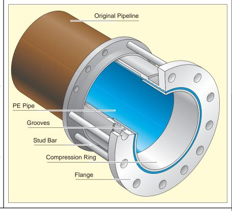
as the yield-strength of the PE is not exceeded, no permanent deformation will occur.
